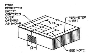
Note: Fastening plates are required at the end laps of the perimeter membrane sheets on both sides of the opened area.
