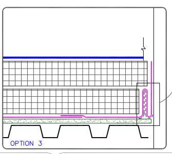
CONTINUOUS STRIPPING OF SELF-ADHERING VAPOR RETARDER 725TR FULLY ADHERED TO WALL AND SUBSTRATE WITH DOUBLE FOLD CREASES MIN. 2" (51mm) HIGH, SET VERTICALLY UP AGAINST THE WALL. DO NOT ADHERE THE FOLDS TOGETHER
