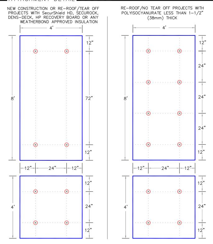
NOTE: FOR CRITERIA ON INSULATION FASTENERS AND PLATES, REFER TO CARLISLE SPECIFICATIONS.
