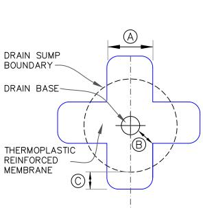
CUT SECTION OF THERMOPLASTIC REINFORCED MEMBRANE AS SHOWN AND POSITION INTO DRAIN SUMP. EXTEND MEMBRANE OUT OF DRAIN SUMP APPROXIMATELY 6" (15cm) (ROUND CORNERS).
