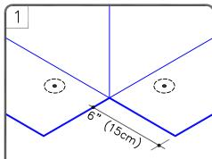
FASTEN MEMBRANE AND FLASH CURB OR WALL WITH CURED EPDM MEMBRANE FOLLOWING STANDARD PROCEDURES USING BONDING ADHESIVE AND PAS SEAM TAPE AT MEMBRANE SPLICE.
