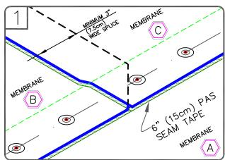
POSITION MEMBRANE TO ALLOW AN APPROXIMATE 7" (17.5cm) OVERLAP ALONG THE LENGTH OF THE MEMBRANE & 4" (10cm) AT END LAPS. THE PRE-MARKED LINE ON THE MEMBRANE EDGE CAN BE USED AS A GUIDE FOR THE TAPE PLACEMENT.
