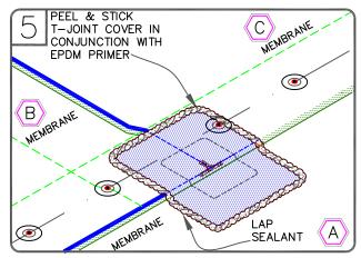
APPLY 6" (15cm) WEATHERBOND PEEL & STICK T-JOINT COVER AND 12" (30cm) PEEL & STICK T-JOINT COVER CENTERED OVER THE INTERSECTING POINT OF THE LEADING EDGES OF THE FIELD SPLICE INTERSECTION AS SHOWN.
