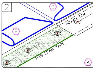
FOLD SHEETS BACK AS SHOWN. APPLY EPDM PRIMER TO THE SPLICE AREA ON BOTH SURFACES AND ALLOW TO PROPERLY DRY. APPLY PAS SEAM TAPE WITH RELEASE FILM ALIGNED WITH MARKER LINE.
