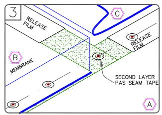
SPLICE SHEET B TO SHEET A AND APPLY SECOND PIECE OF PAS SEAM TAPE BETWEEN SHEET B AND C. TRIM RELEASE FILM AS SHOWN.
