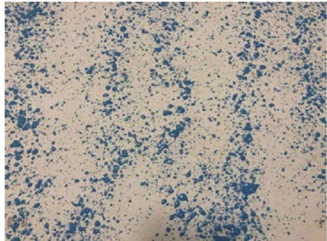
FIG 2. LIGHT COVERAGE – SPLATTER APPLICATION
