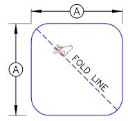
CUT A SECTION OF WEATHERBOND THERMOPLASTIC NON-REINFORCED MEMBRANE WITH ROUNDED CORNERS
