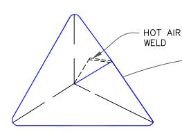
POSITION AND HEAT WELD CORNER IN PLACE AS SHOWN
