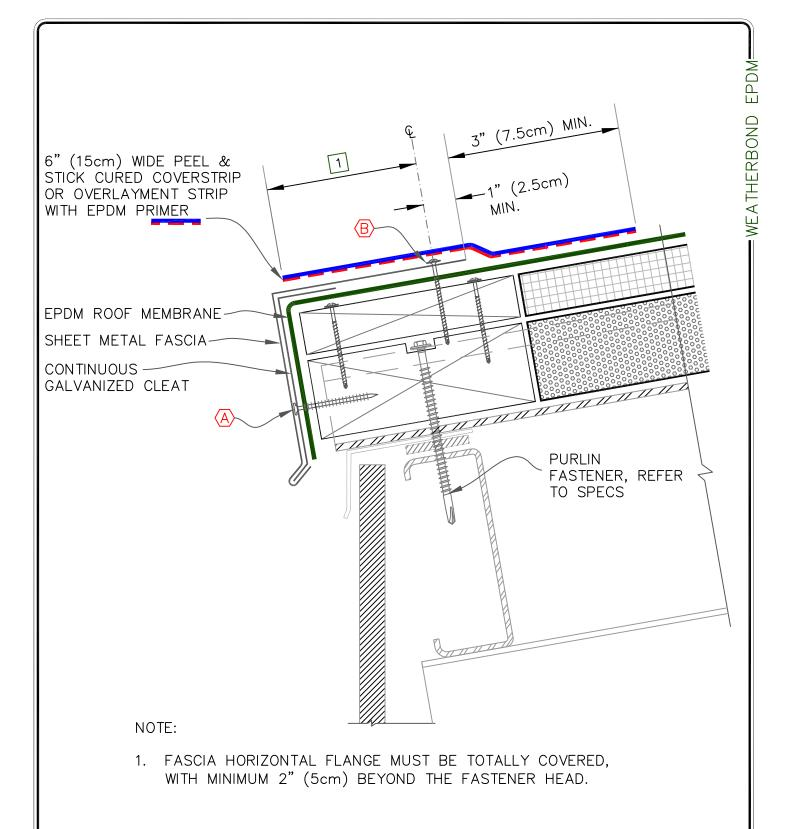
△ 1-1/2" (38mm) RING SHANK NAILS @ B HPW FASTENERS @ 12" (30cm) O.C. 6" (15cm) O.C. MAXIMUM
