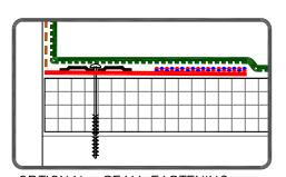
OPTIONAL: SEAM FASTENING PLATE/FASTENER MAY BE INSTALLED INTO THE STRUCTURAL DECK ALSO.
