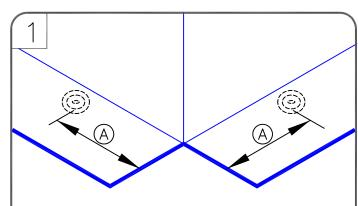
FASTEN MEMBRANE AND FLASH CURB OR WALL WITH CURED EPDM MEMBRANE FOLLOWING STANDARD PROCEDURES USING BONDING ADHESIVE and PAS SEAM TAPE.
