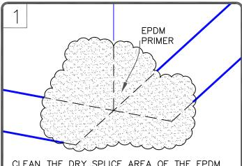
CLEAN THE DRY SPLICE AREA OF THE EPDM MEMBRANE BY SCRUBBING WITH EPDM PRIMER.
