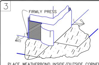
PLACE WEATHERBOND INSIDE/OUTSIDE CORNER AS SHOWN AND REMOVE RELEASE PAPER. PRESS FOLDED FLASHING TIGHTLY INTO ANGLE CHANGE AND FIRMLY PRESS FLASHING AGAINST THE VERTICAL SURFACE.
