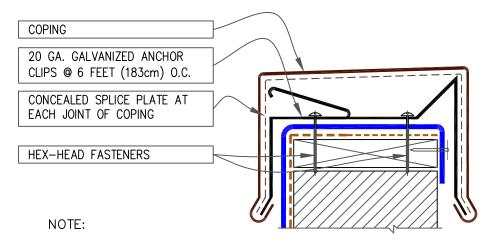
1. MEMBRANE MUST BE EXTENDED AT CORNERS TO PROVIDE COMPLETE COVERAGE OF THE TOP WALL SURFACE. REFER TO DETAIL WBRC-9.0B.
