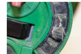
DIRT AND DEBRIS IN INTAKE
