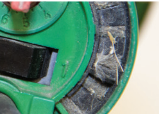
DIRT AND DEBRIS IN INTAKE
