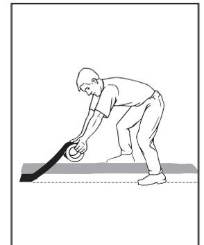
Unroll 3"-wide white EPDM Seam Tape along the length of the seam, tape side down, and align the Seam Tape (not the clear backing) along the chalk line. Using moderate pressure, set the Seam Tape into place to avoid air entrapment. Fold the top membrane onto the Seam Tape release paper. (If the Seam Tape does not visibly extend beyond the leading seam edge, the membrane should be repositioned to expose one quarter inch (¼) of Seam Tape.)
