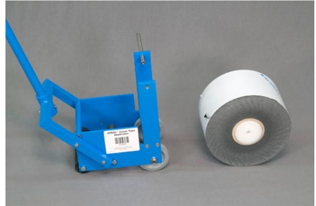
4. Using hands, pull cover tape down through applicator with the sticky side down. Pull tape beneath the gray roller and position under the 6 segmented pressure wheels as shown and begin applying.
