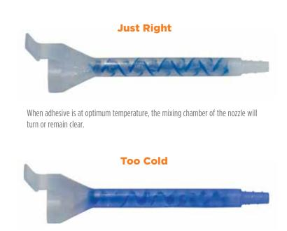
The entire tip will be blue when cold adhesive is sprayed through it. Stop spraying to avoid off-ratio adhesive and properly condition the tanks before spraying again.
