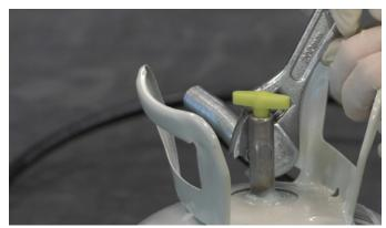
Step 3: Connect the hose to the UN-TACK cylinder using an openend or adjustable wrench. Once securely attached, open the valve on top of the UN-TACK cylinder.
