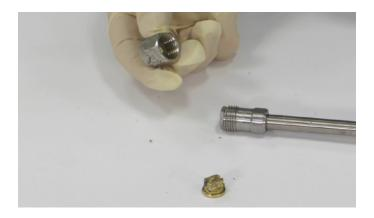
**Step 3:** Place a new spray tip or cleaned spray tip into the retaining cap. Turn the retaining cap onto the threaded extension assembly.
