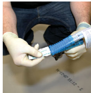
Application of petroleum jelly to spray gun
