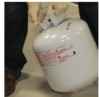
Shaking of A-side and B-side tanks
