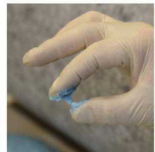
Performing the string-time test
