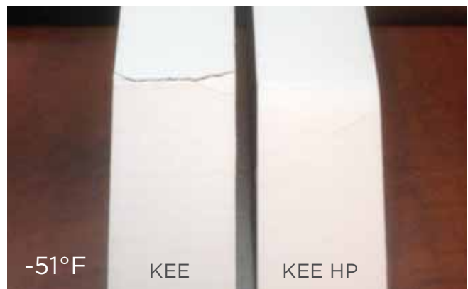
Same formulation except for the upgrade from standard KEE to KEE HP
